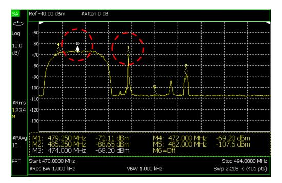
Observe the difference between maximum amplitude of the video carrier of the TV signal (1) and the max amplitude of WSD (3)
